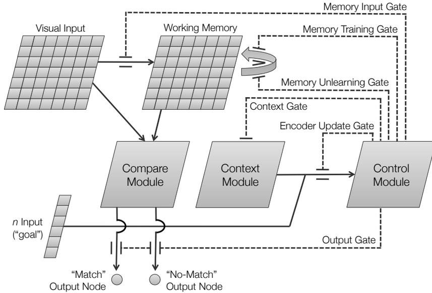
**Figure 1.** The GALIS model as used for the  $n$ -Back task. Thin, solid arrows denote one-to-one connections. The working memory layer is fully recurrently connected (broad arrow). Dotted lines are the outputs of the control module. Note that the number of boxes pictured in each layer is an approximation only, and does not faithfully represent the number of nodes used in the model.
