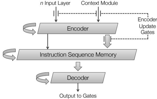
**Figure 2.** Slightly expanded control module showing its gated input encoder and output decoder which function as heteroassociative memories.
