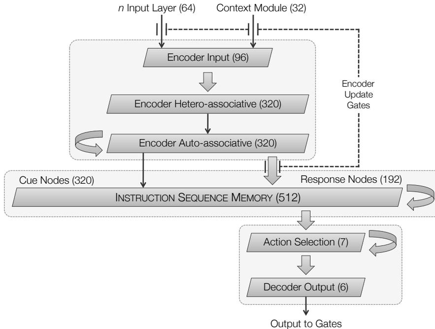
**Figure A.8.** The control module. Thick arrows denote fully connected layers, while thin arrows denote one-to-one connections. Following the name of each layer is the number of nodes it contains in the example presented in this paper. One-to-one connections from the Encoder Auto-associative layer terminate on the cue nodes of the instruction sequence memory, while full connections terminate on the response nodes.
